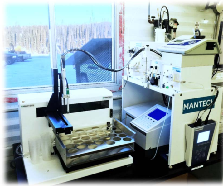
MT-100 performing pH, EC, Alkalinity, Turbidity, Colour, and Ammonia at a Remote Mine Site
