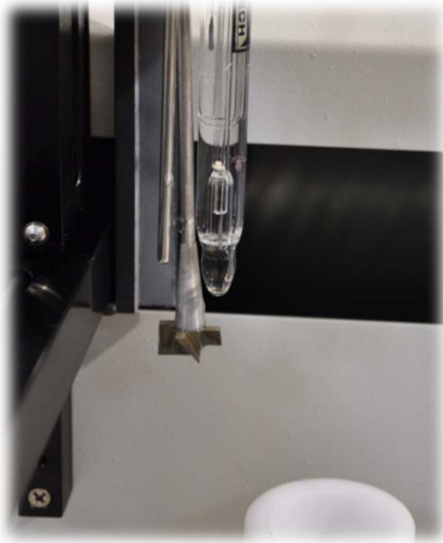
Powerful, baffled soil stirrer
